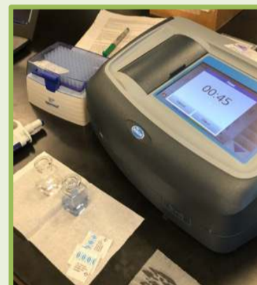
Measuring extractable phosphate
