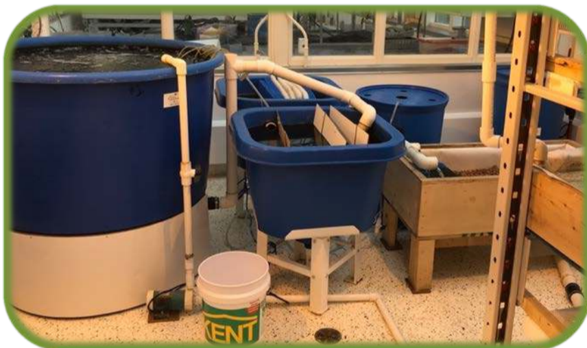
Figure 2. Fish tank and filtration tanks
